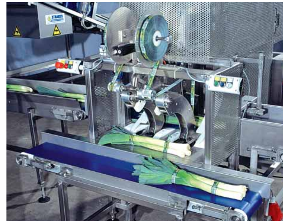
The newly designed banded unit bunches the weighed leek packages by two adhesive tapes
