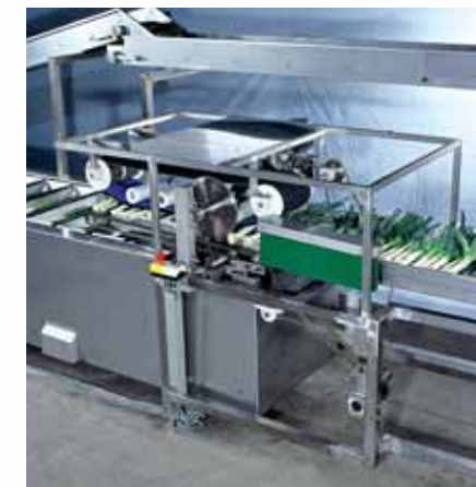
The product is adjusted variably, held to the position by a holding-down device and cut by a special knife on the the root- and leaf side of the leek.
