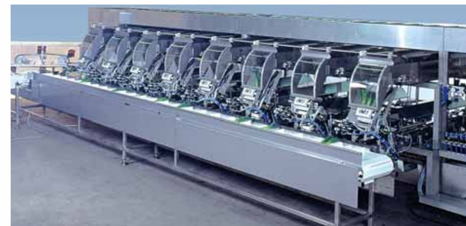
The weighed leek arrangements are transported from the cross belts into the insertion robots. The erected cardboard bowls are transferred from the magazine. Finally, the leek is feeded into the bowls by opening the baffle.
