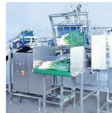
The leek box dumper as a fully automatic and product sparing draining facility.
